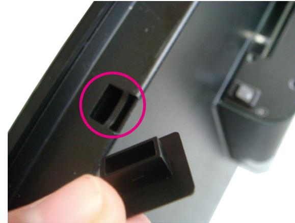
2. Insert the hole block into the opening until it is pushed in completely.
