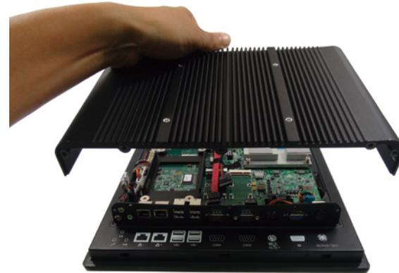
2. Remove the mounting screws on the metal support plate.
