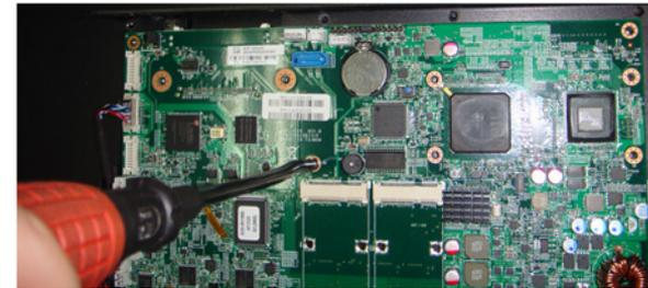
3. The SATA DOM package includes a supporting stud. The stud is used to stabilize the SATA DOM module.
