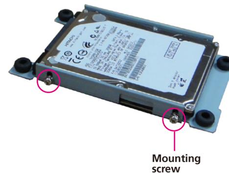
6. Place the SATA drive in the chassis and then use the provided mounting screws to secure the drive in the chassis.
