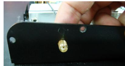
7. Insert the ring onto the antenna jack end of the cable.
